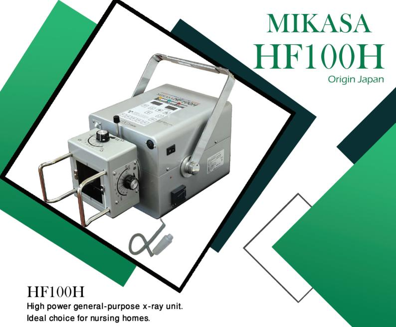
The HF100H is compact and lightweight enabling easy transportation. It is capable of taking exposures of most body parts using maximum 100 kV and maximum 40mA high frequency technology. The unit has 5 memory stations for storing x-ray exposure techniques. It is compatible with all major DR digital systems. It is recommended for hospitals, mobile clinics, military field clinics and nursing homes.
